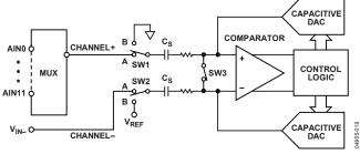
Figure 45. ADC in Pseudo Differential Mode
