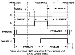
Both switching edges are moved by an equal amount (*PWMDAT1* ×  $t_{CORE}$ ) to preserve the symmetrical output patterns.
