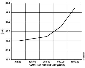
Figure 32. Current Consumption vs. Sampling Frequency
