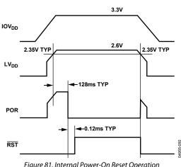
Figure 81. Internal Power-On Reset Operation
