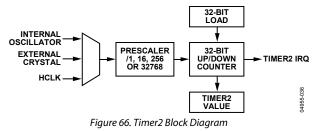
Timer2 interface consists of four MMRs: T2LD, T2VAL, T2CON, and T2CLRI.
