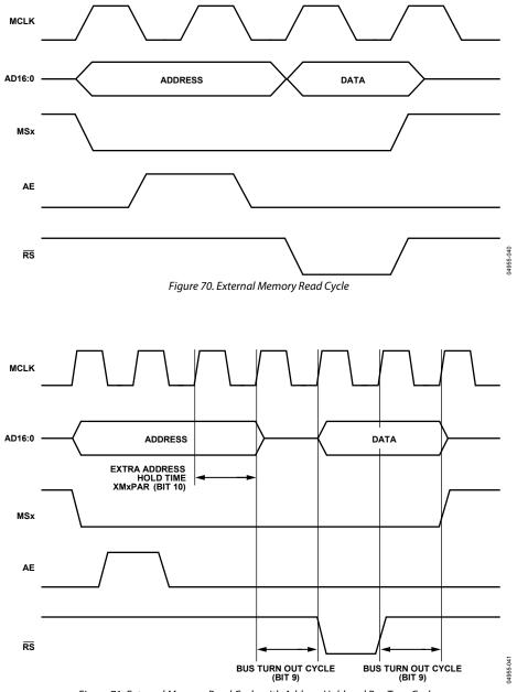
Figure 71. External Memory Read Cycle with Address Hold and Bus Turn Cycles
