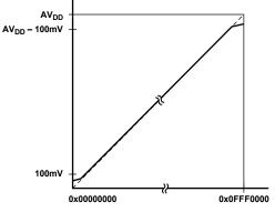
Figure 53. Endpoint Nonlinearities Due to Amplifier Saturation
