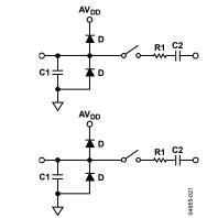
Figure 47. Equivalent Analog Input Circuit Conversion Phase: Switches Open, Track Phase: Switches Closed
