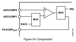
Note that because the ADuC7022, ADuC7025, and ADu7027 parts do not support a DAC0 output, it is not possible to use DAC0 as a comparator input on these parts.
