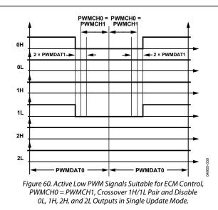
In addition, the other four signals (0L, 1H, 2H, and 2L) have been disabled by setting the appropriate enable/disable bits of the PWMEN register. In Figure 60, the appropriate value for the PWMEN register is 0x00A7. In normal ECM operation, each inverter leg is disabled for certain periods of time to change the PWMEN register based on the position of the rotor shaft (motor commutation).
