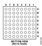
Figure 16. 64-Pin BGA Pin Configuration (ADuC7028)
