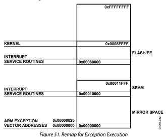
By default, and after any reset, the Flash/EE is mirrored at the bottom of the memory array. The remap function allows the programmer to mirror the SRAM at the bottom of the memory array, which facilitates execution of exception routines from SRAM instead of from Flash/EE. This means exceptions are executed twice as fast, being executed in 32-bit ARM mode with 32-bit wide SRAM instead of 16-bit wide Flash/EE memory.
