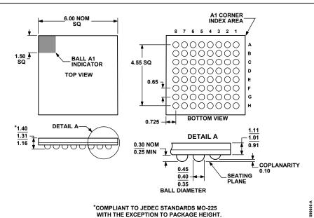
\*COMPLIANT TO JEDEC STANDARDS MO-225 WITH THE EXCEPTION TO PACKAGE HEIGHT. Figure 87. 64-Ball Chip Scale Package Ball Grid Array [CSP\_BGA] (BC-64-4) Dimensions shown in millimeters
