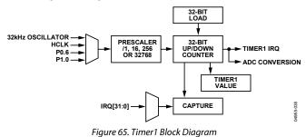
Timer1's interface consists of five MMRs: T1LD, T1VAL, T1CON, T1CLRI, and T1CAP.
