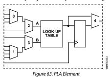
In total, 30 GPIO pins are available on each ADuC7019/20/21/ 22/24/25/26/27/28 for the PLA. These include 16 input pins and 14 output pins, which need to be configured in the GPxCON register as PLA pins before using the PLA. Note that the comparator output is also included as one of the 16 input pins.
