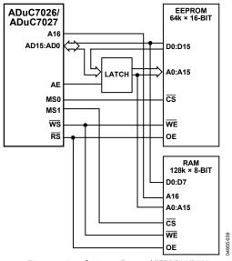
Figure 69. Interfacing to External EEPROM/RAM
