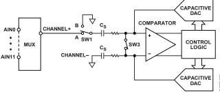
Figure 46. ADC in Single-Ended Mode
