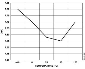
Figure 30. Current Consumption vs. Temperature @ CD = 7
