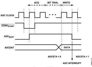
Figure 41. ADC Timing
