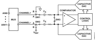
Figure 43. ADC Acquisition Phase
