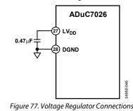
The LV\_{DD} pin should not be used for any other chip. It is also recommended to use excellent power supply decoupling on  $IOV_{DD}$  to help improve line regulation performance of the on-chip voltage regulator.
