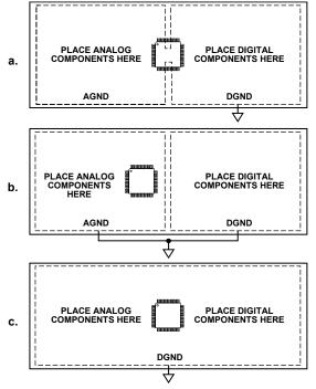
Figure 78. System Grounding Schemes
