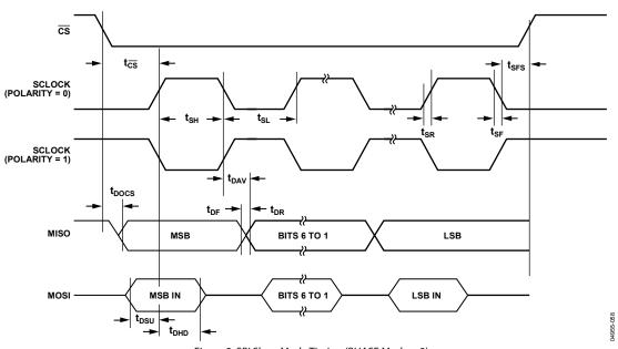
Figure 9. SPI Slave Mode Timing (PHASE Mode = 0)
