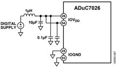
Figure 76. Recommended IOV<sub>DD</sub> Supply Filter
