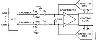
Figure 44. ADC Conversion Phase
