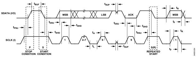
Figure 5. I<sup>2</sup>C Compatible Interface Timing
