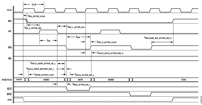
Figure 3. External Memory Write Cycle
