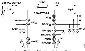
Figure 75. External Single Supply Connections
