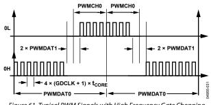
Figure 61. Typical PWM Signals with High Frequency Gate Chopping Enabled on Both High-Side and Low-Side Switches
