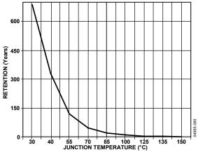
Figure 50. Flash/EE Memory Data Retention
