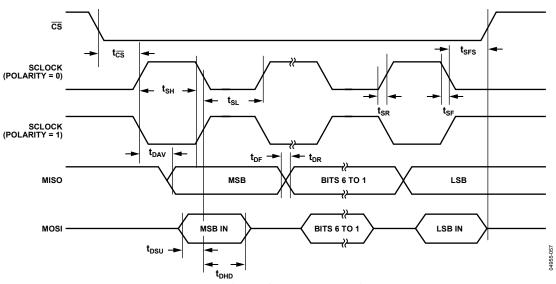
Figure 8. SPI Slave Mode Timing (PHASE Mode = 1)
