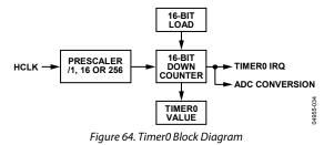
Timer0's interface consists of four MMRs: T0LD, T0VAL, T0CON, and T0CLRI.
