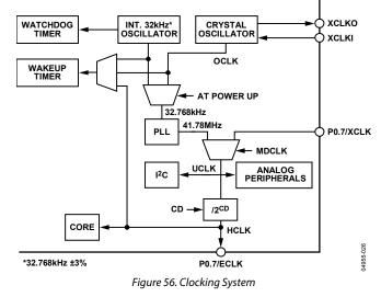
The selection of the clock source is in the PLLCON register. By default, the part uses the internal oscillator feeding the PLL.
