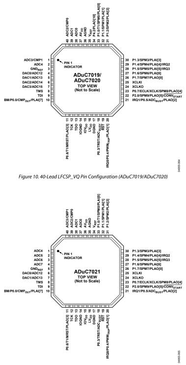
Figure 11. 40-Lead LFCSP\_VQ Pin Configuration (ADuC7021)
